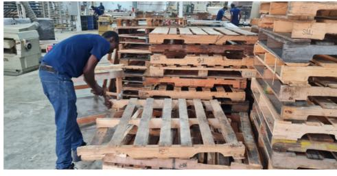
A member of staff in our Manufacturing & Recycling Division repairs a damaged pallet
