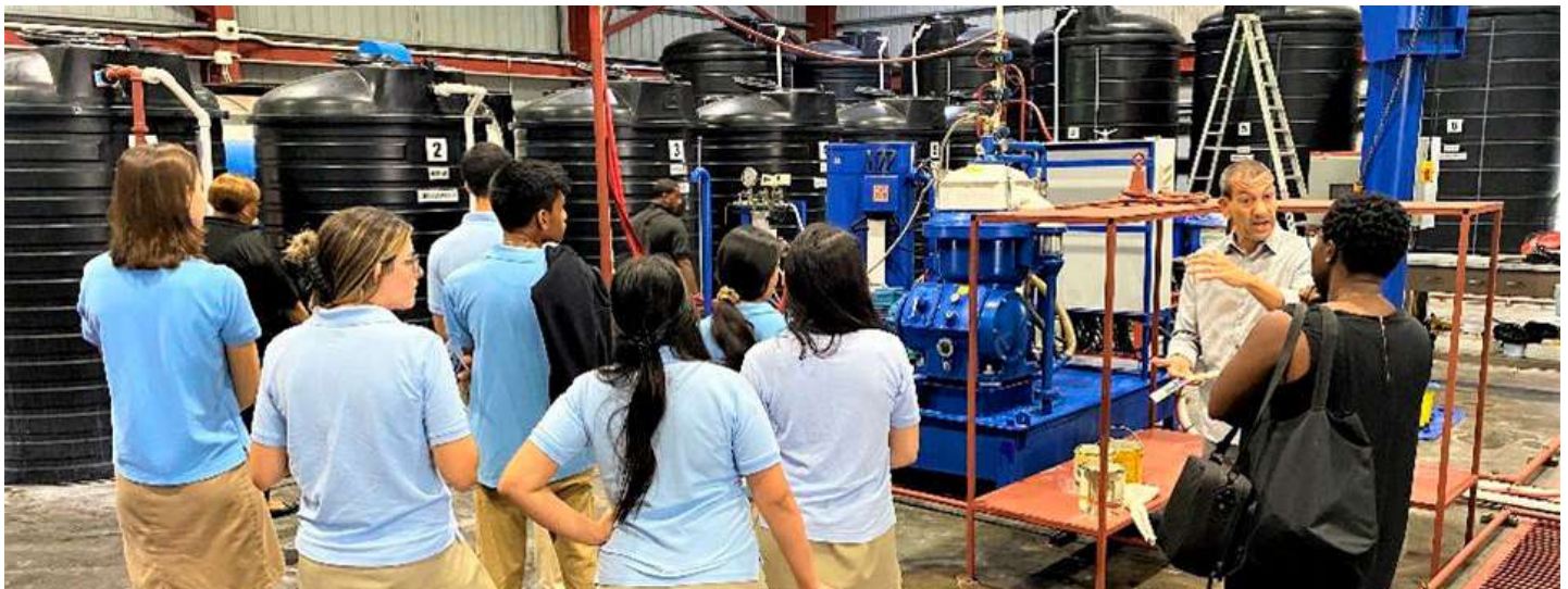
Kevin Whiteman, Managing Director of HADCO's Recycling Division explains how the centrifuge works in the process of recycling WVO
