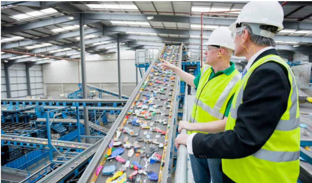
Crushed plastic PET bottles on a conveyor belt in an EU recycling plant Image Credit: plasticseurope.org
