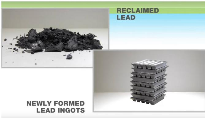
The scrap lead material is taken to a furnace and alloyed into ingot bars.
