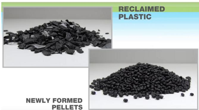
The plastic is reclaimed by a cleaning and melting process that transforms the crushed pieces into finer pellets.
